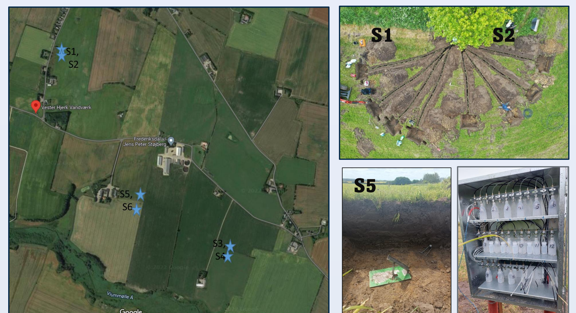
Fig. 2. Overview of the six monitored fields (S1-S6) located near Skive, Denmark, representing different cropping systems. The photos show site layout, installation of 8 suction cells at 1 m depth per site/field, and the water sampling.
