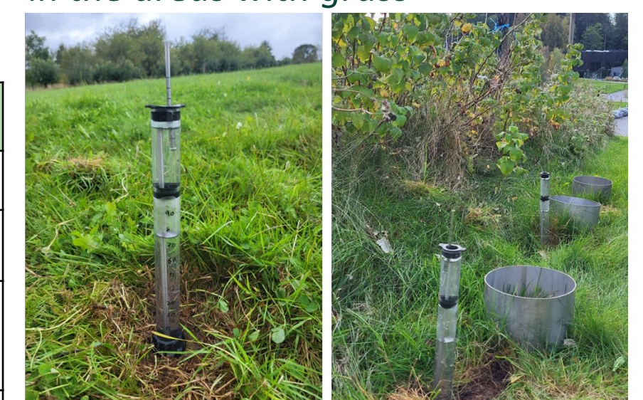
Figure 3. Infiltration test: minidis (soil matrix infiltration) & single ring method with the Beerkan approach (total infiltration)
