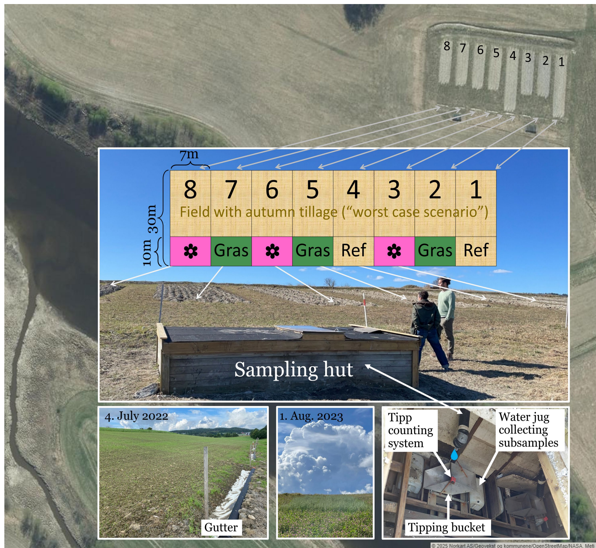
Figure 1. Experimental set-up. Aerial photo of the test field, with the eight plots and two sampling-huts. The vegetation in the eight plots are illustrated (gras: green, flowers: pink, and reference (cereal): yellow.). Pictures of the test-field and sampling-system.
