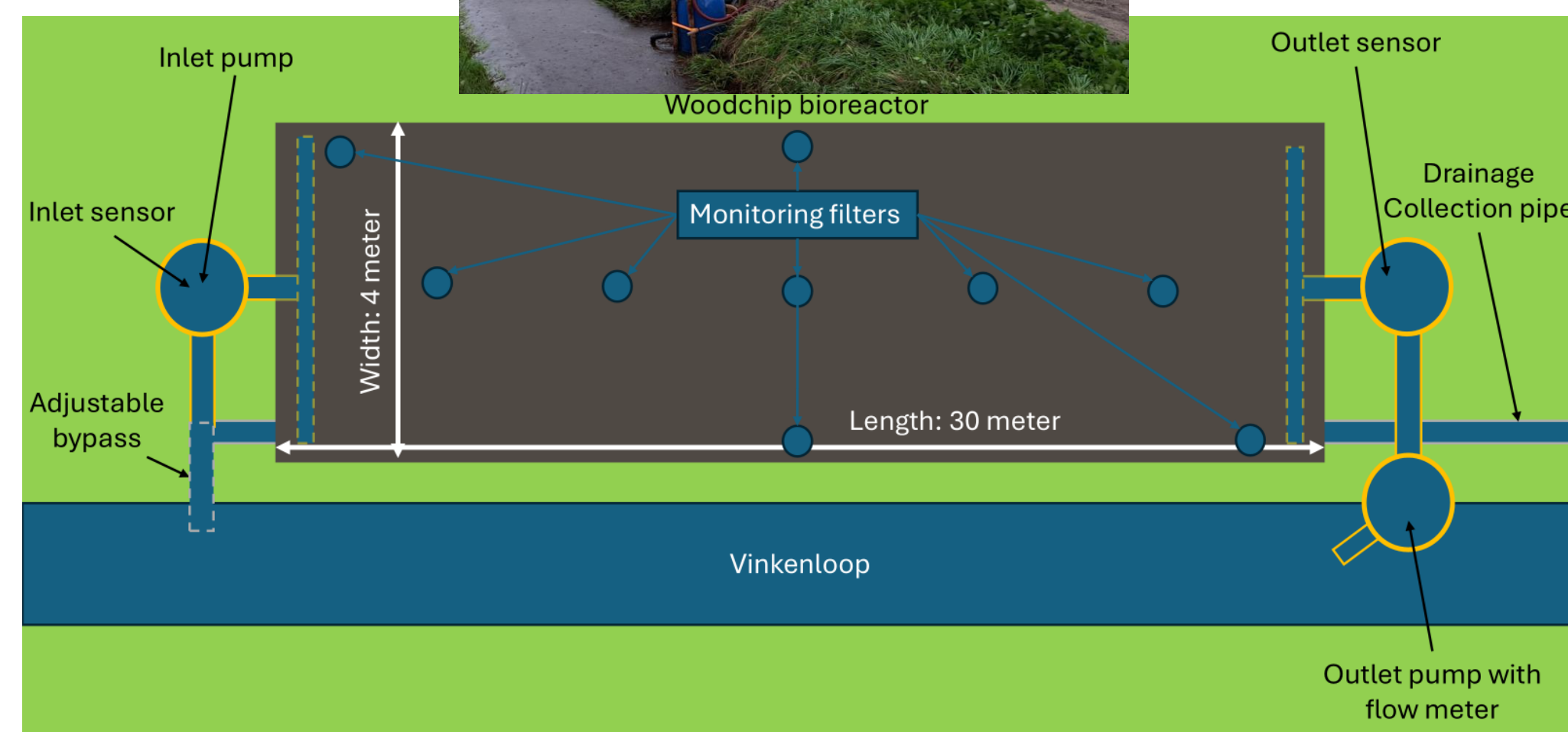
Figure 2: Schematic overview and picture of the developed woodchip bioreactor in the South of the Netherlands.
