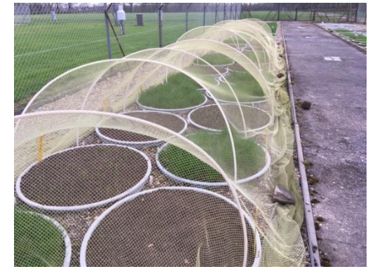
Test period 2 yrs: (1) Fertilized grass (2) Vegetation free (3) Spring barley (4) Spring barley + CC
